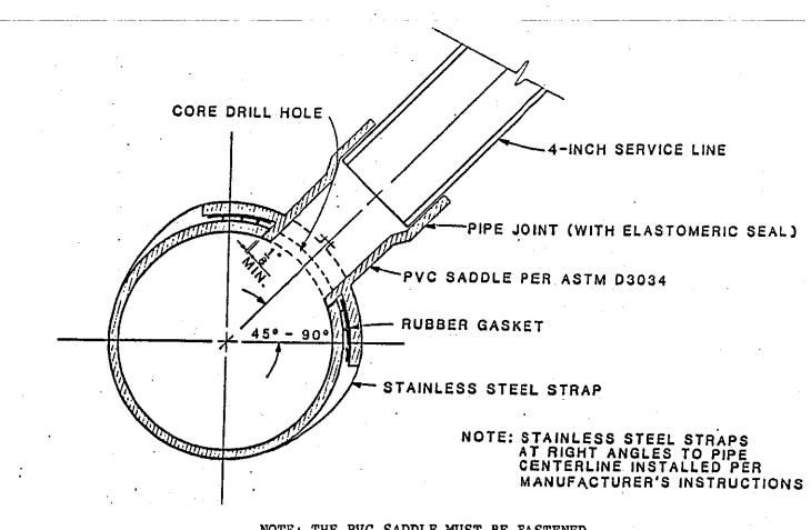
NOTE; THE PVC SADDLE MUST BE FASTENED TO THE MAIN USING EPOXY IN ADDITION TO THE STEEL STRAPS.
